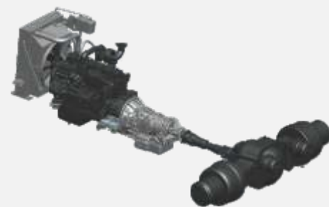
Renounced & reliable drive line Cummins engine+ Allison Transmission+Meritor Fabricated design axle.
